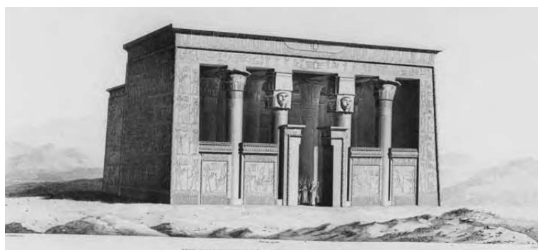
Plate 120 Plate from Description, A, Vol. I , showing the elevation of the portico of the great temple at Edfu (otherwise known as Apollonopolis Magna). Note the three types of capital and the pluteus (GB/SM).
